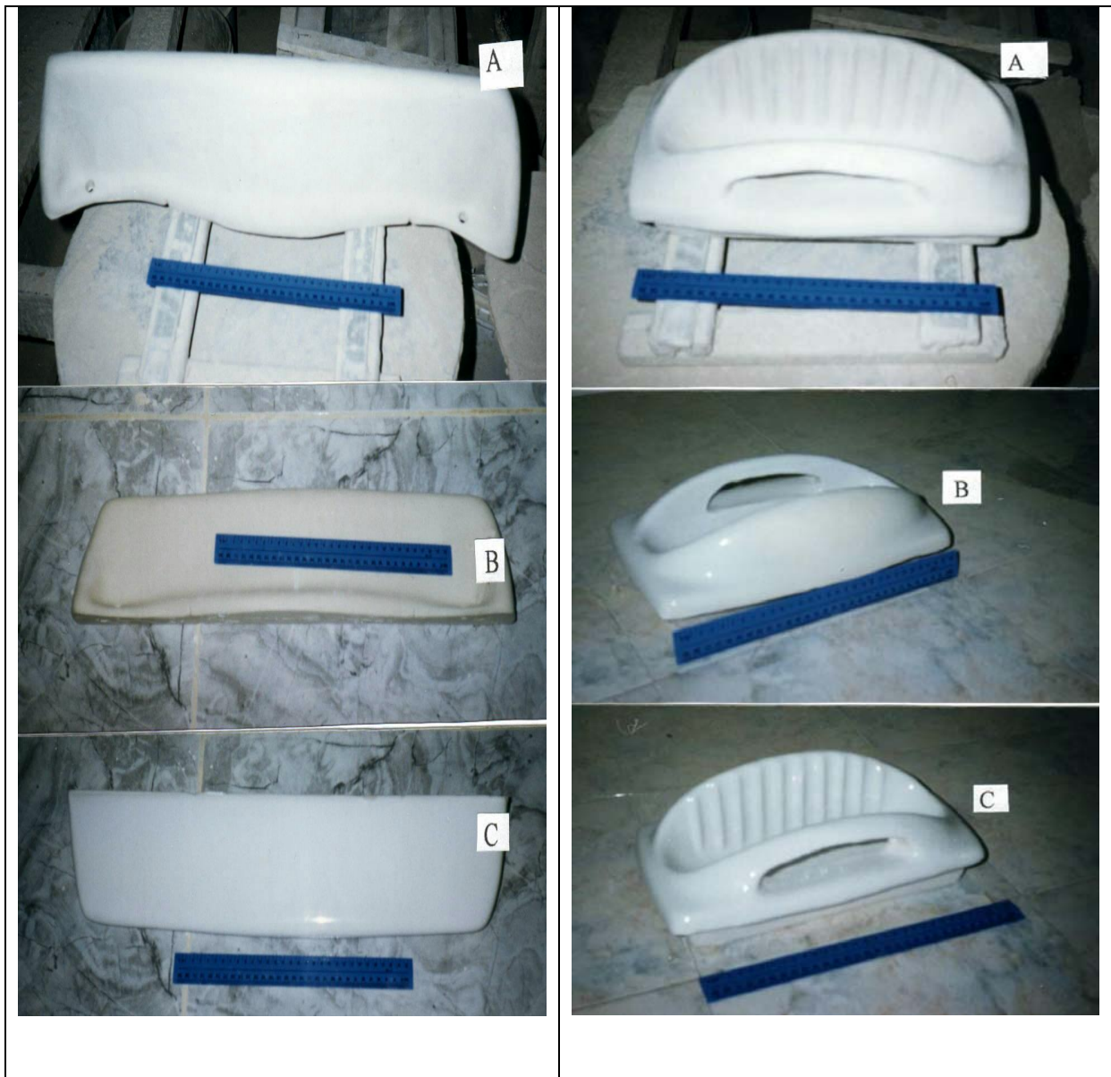
Figure (5): The Sanitaryware Article: a) Before firing; b) After firing without glazing; c) After firing with glazing materials.
