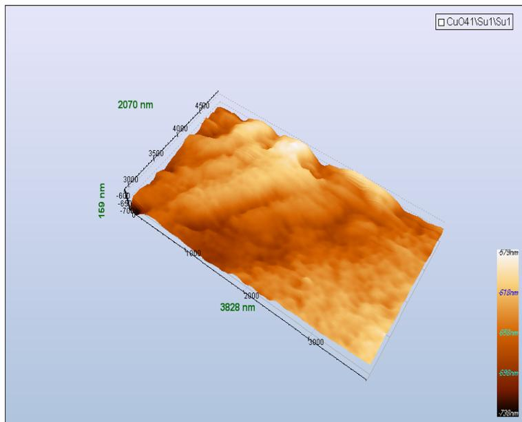
Fig. 2. Topographic image of Copper oxide nanoparticles by STM
