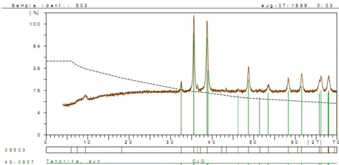
Fig. 3. XRD pattern of Copper oxide nanoparticles
