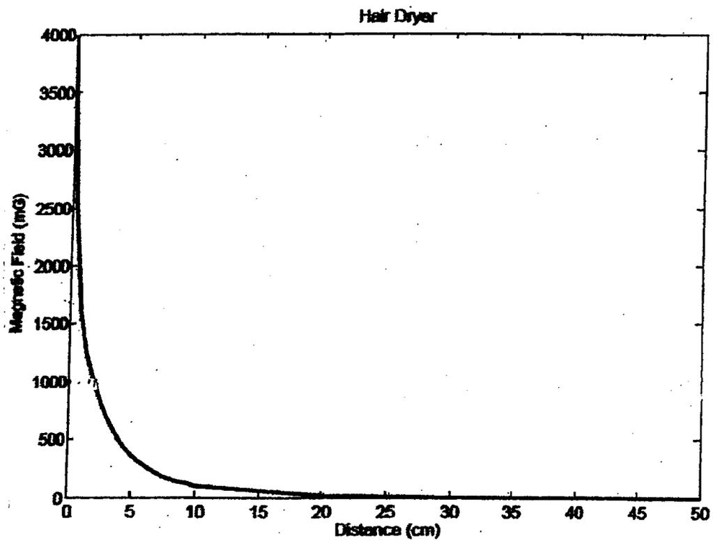
Fig. 5.1: Electric and magnetic fields Vs. Distance from a hair dryer
