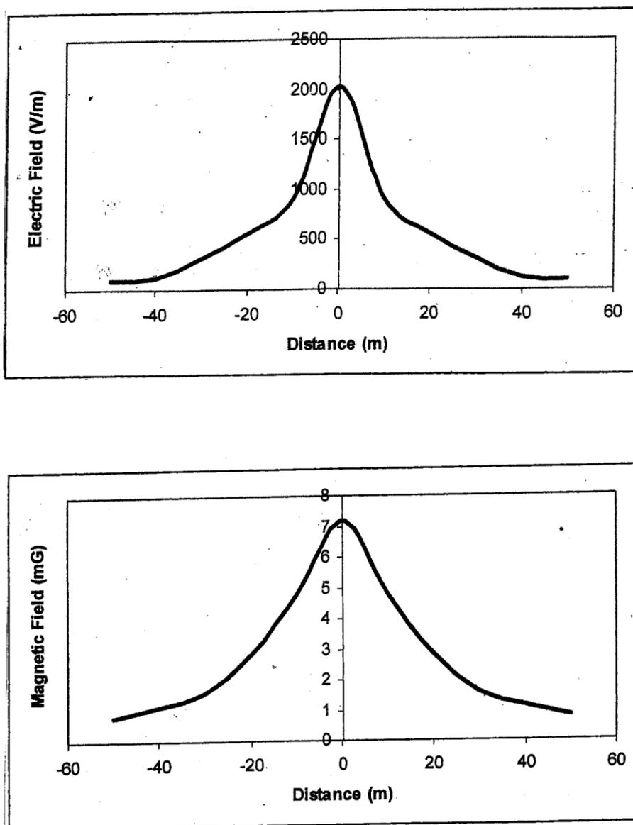
Fig. 5.2: Electric and magnetic fields Vs. Distance from the centerline of the 400 KV South Amman – East Amman OHL.
