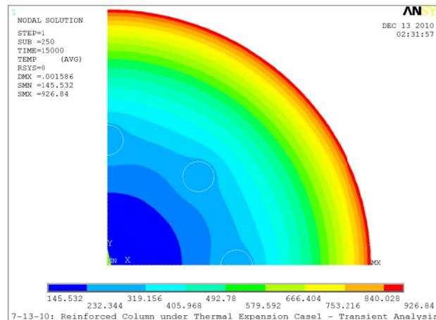
**Figure 5: Temperature Distribution Through Cross-Section of Column**
