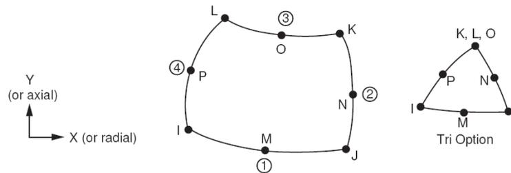
Figure 3: Plane223 Geometry
