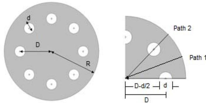
Figure 2: (a) Cross Section (b) RVE of Column
