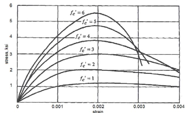
Figure 1: Typical Concrete Stress-Strain Curves (1 ksi = 6895 kPa), (McCormac 2008)
