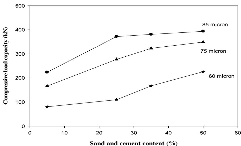
**Figure 1. The influence of sand and cement content (%) on the compressive load capacity of the composite used in this study for the cooling rate of  $12^{\circ}C/min$ .**
