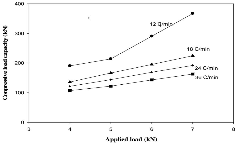
Figure 2. The influence of applied load on the compressive load capacity of the composite used in this study for particle size of 85 micron
