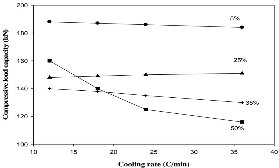
Figure 3. The influence of cooling rate on the compressive load capacity of the composite used in this study
