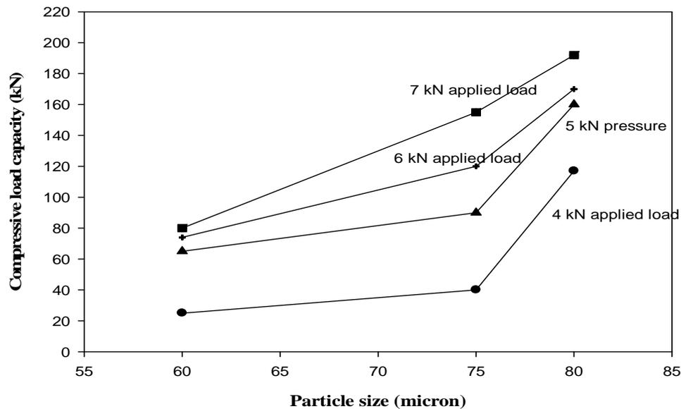
**Figure 4. The influence of particle size on the compressive load capacity of the composite used in this study**
