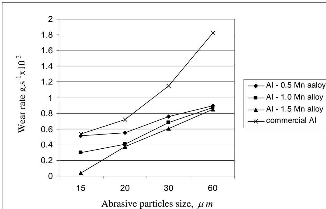
**Fig. 10 Effect of abrasive particles size on wear rate.**
