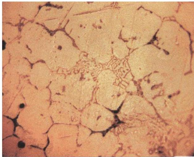
**Fig. 8 Microstructure of Al-1.0Mn alloy (40X).**
