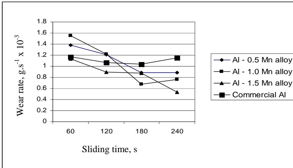
Fig. 1 Effect of sliding time on wear rate.
