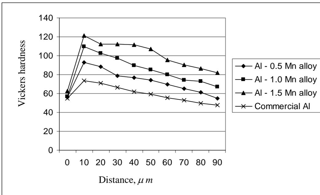
Fig. 4 Vickers hardness (from surface to center) at minimum load 0.45N and time 120s.
