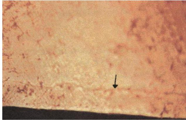
Fig. 5 Effect of maximum load on surface damage and layer of material removal of Al-1.5Mn alloy (40X).
