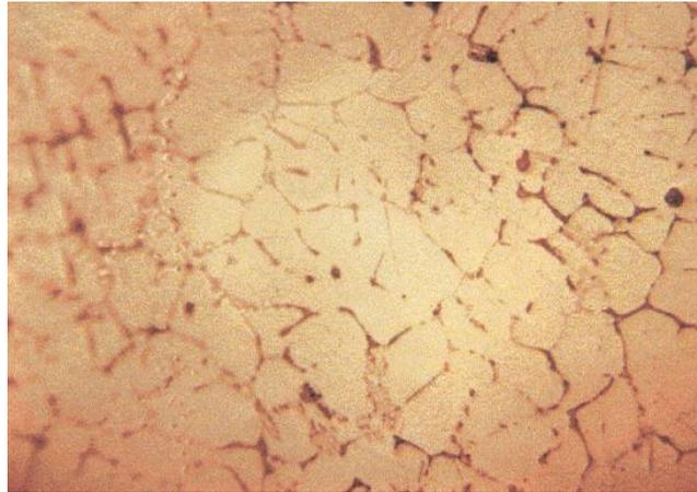
**Fig. 7 Microstructure of Al-0.5Mn alloy (20X).**
