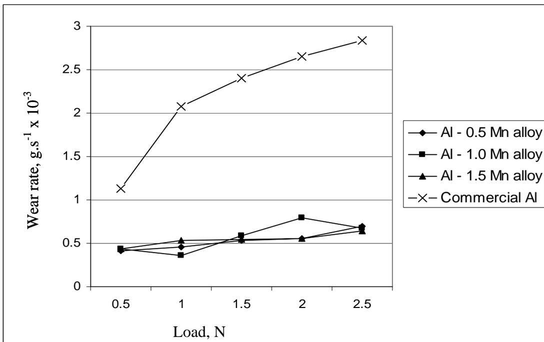
Fig. 2 Effect of load on wear rate.
