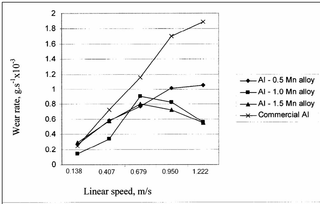
Fig. 6 Effect of linear speed on wear rate.
