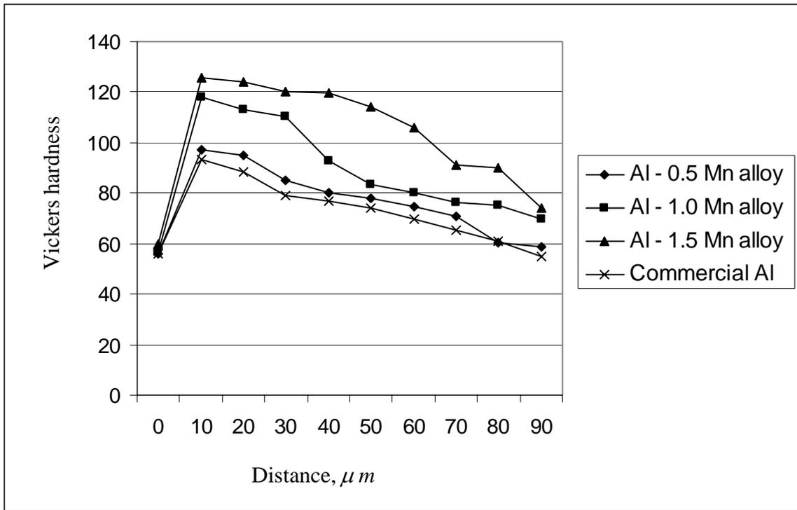
Fig. 3 Vickers hardness (from surface to center) at maximum load 2.45N and time 120 s.
